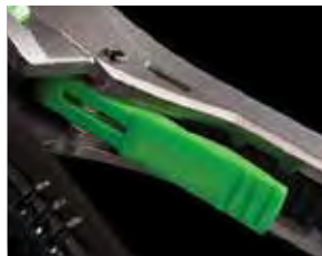
A QUICK-RELEASE BUTTON ALLOWS YOU TO FREE THE TUBE WITH EASE AND WITHOUT DAMAGE.
