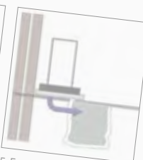
5. For floor-mounted ASHP fit the pipework from the ASHP into the soakaway bag
