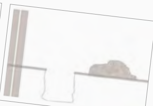
3. Dig a hole minimum 500mm deep x minimum 400mm diameter.
