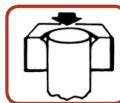
**SELF GAUGING** - Just insert tube flush with top of die for accurate flare size.
